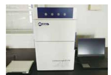
LuminoGraph II EM with F0.8 ultra-sensitive lens and ultra-low noise EM CCD camera allows to detect chemiluminescence and fluorescence signal from Western blot membranes and SDS-PAGE gels. Four LEDs (Blue, Green, Red, NIR) and white transilluminator are equipped.
