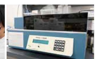
P-2000 micropipette puller (Sutter) is equipped with a CO<sub>2</sub> laser-based heat source and can manufacture quartz glass pipettes. Quartz glass has extremely high physical strength and can achieve a tip diameter of 0.01 micron or less, which is not possible with ordinary glass. In addition, the CO<sub>2</sub> laser is not easily affected by the external environment such as temperature and humidity, and has high reproducibility.
